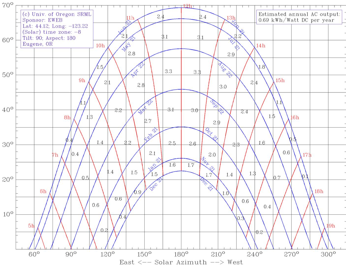
The sun path chart to the right is for a solar electric system located in Eugene, Oregon tilted 90 degrees with a 180 degree azimuthal orientation. The annual AC output for a system with these characteristics is about 0.69 kWh/Watt DC per year.
