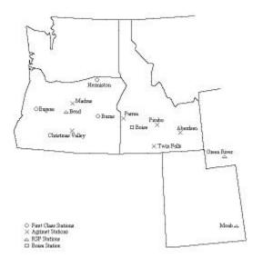
Fig. 1: UO Solar Monitoring Network. Open circles  $(\bigcirc)$  indicate stations containing both global and beam solar instrumentation. AgriMet stations are labeled (X). Global and diffuse irradiance are measure at AgriMet stations. Triangles  $(\triangle)$  show the location of RSP stations. RSP stations measure global and diffuse radiation and calculate beam radiation. The Boise station has both an RSP and AgriMet instrumentation and is labeled with a square  $(\Box)$ .
