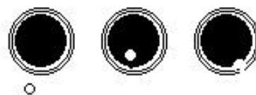
Fig. 19: Spot of light moves across PSP sensor.
