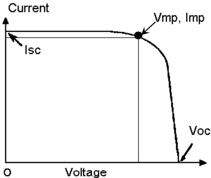
Plot of IV curve for a solar cell. Current times Voltage equals Power. Short circuit current (the current when the voltage is zero) increases in proportion to the incident energy (sunlight).
