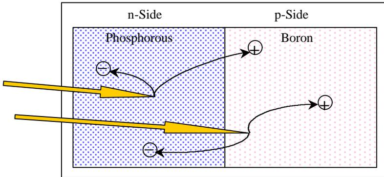
When sunlight striking a cell creates charge carriers (electrons and holes), the electric field pushes new electrons to one side of the junction and new holes to the other. This sorting-out process is what drives the charge carriers in an electric circuit.
