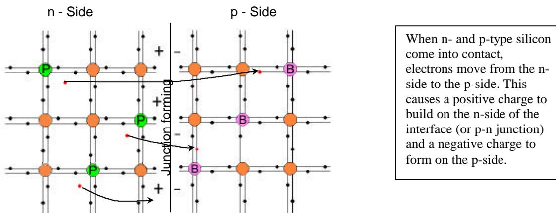
A solar battery is created when n and p type silicon are placed next to each other. The extra electrons from the phosphorous are attracted to the holes created by the doping of the silicon with boron. This occurs because binding of the electron pairs is much stronger than the electromagnetic attraction between the outer electrons and the nucleus of the atoms that is masked by the electrons that are surrounding each atom in the crystal structure.
