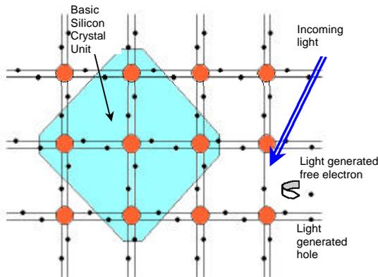
Light of sufficient energy can dislodge a negative electron from its bond in the crystal, creating a positive hole (a bond missing an electron) and a free electron. These negative and positive charges, which move freely for a time about the crystal lattice, are the constituents of electricity.
