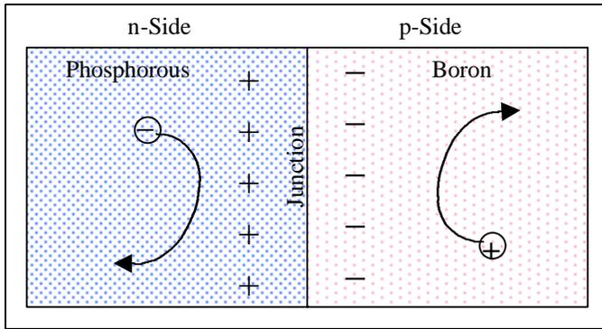
The buildup of excess positive and negative charges on either side of the junction creates an electric field across the interface; the strength of this field depends on the amount of dopant in the silicon. At equilibrium, the electric field repels any additional crossover of holes from the p-side or electrons from the n-side.
