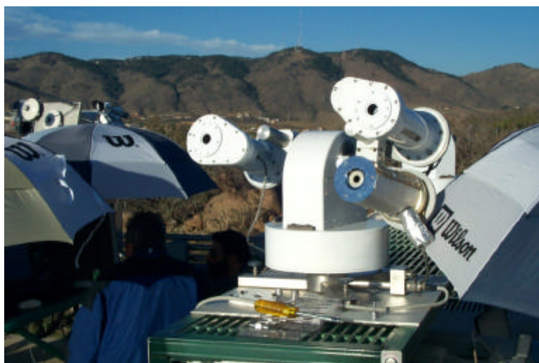
Cavity radiometers at the 2002 NREL Pyrheliometer Intercomparison
