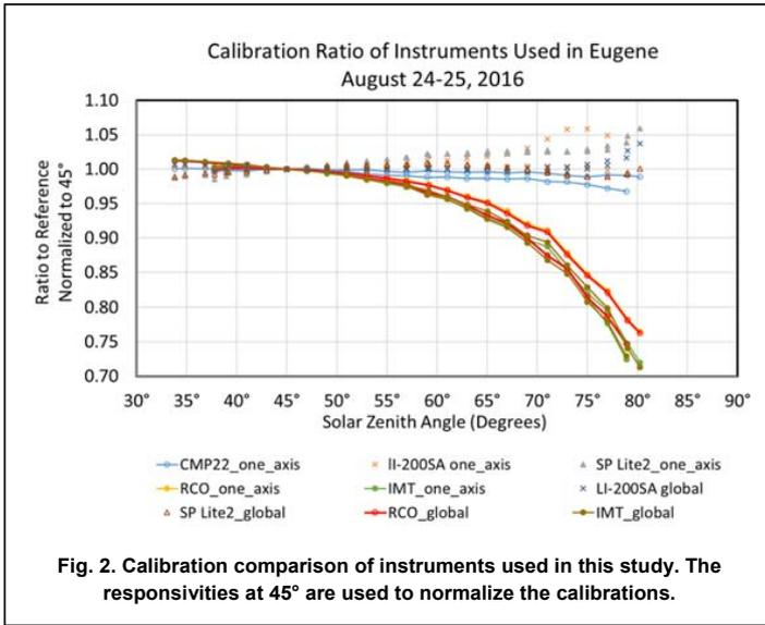
Fig. 2. Calibration comparison of instruments used in this study. The responsivities at 45° are used to normalize the calibrations.
