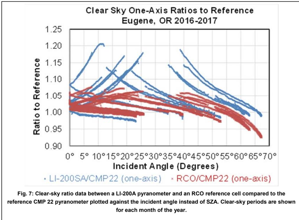
Although the spectral response of the photodiode-based pyranometers and reference cells are similar, they are not identical. The diffuser on the photodiode-based pyranometers has a different spectral response than the glazing on the reference cells.
