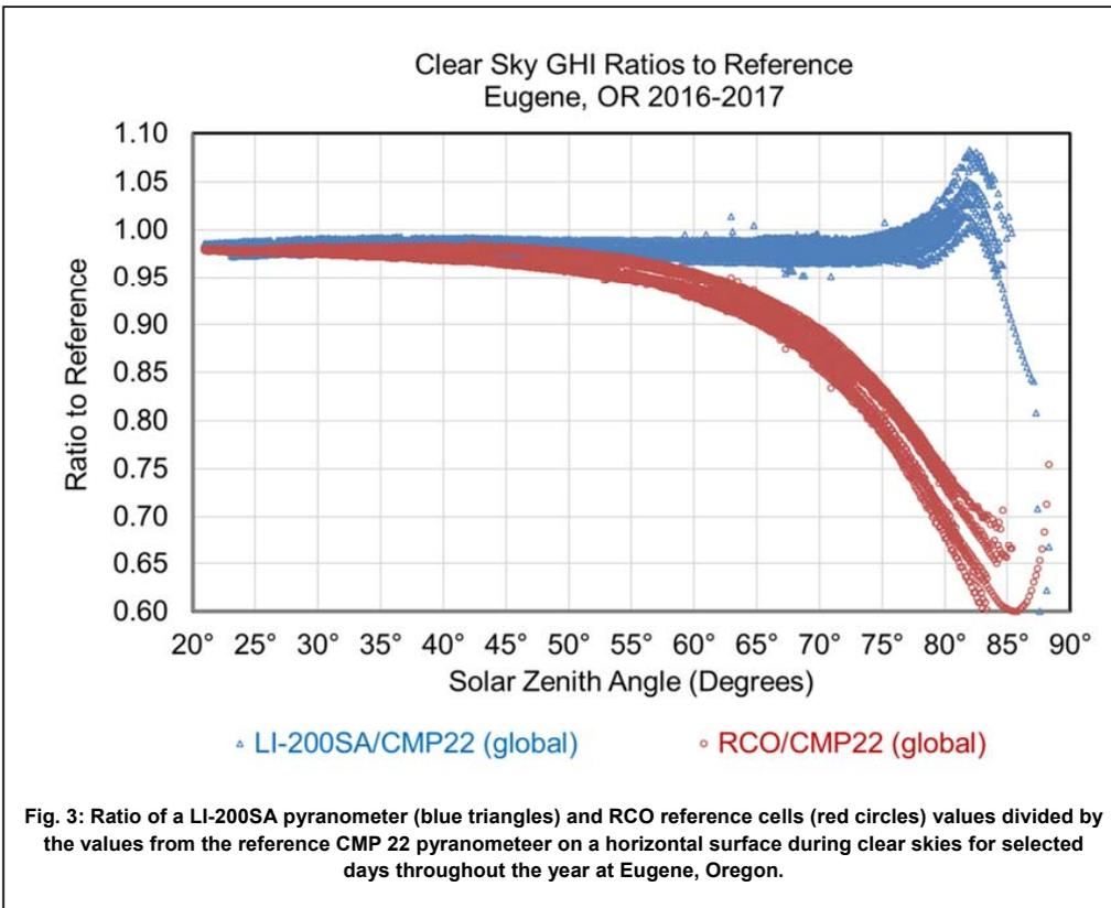
Fig. 3: Ratio of a LI-200SA pyranometer (blue triangles) and RCO reference cells (red circles) values divided by the values from the reference CMP 22 pyranometer on a horizontal surface during clear skies for selected days throughout the year at Eugene, Oregon.
