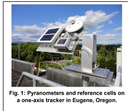
Fig. 1: Pyranometers and reference cells on a one-axis tracker in Eugene, Oregon.
