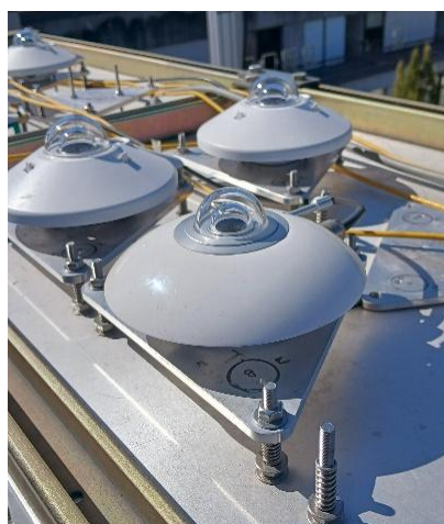
Figure 11. Pyranometers mounted for calibration. Note the mounting platforms used to easily level the sensors.
