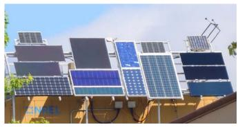
Fig. 1: The NREL PV test facility in Eugene. Picture shot from the lower room and these trees do not shade the modules. The unwashed module is in the upper right hand corner in front of the automatic tracker that can be seen in the background.
