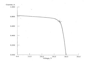
Fig. 2: Performance of unwashed Solarex PV module
