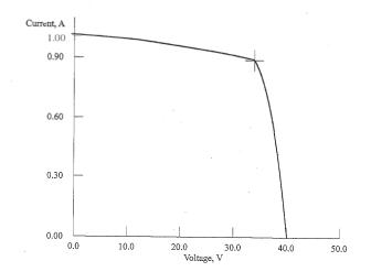
Fig. 3: Performance of Solarex PV module after it was washed.
