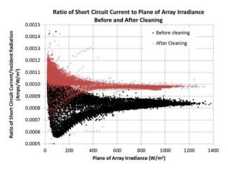
Fig. 4: Plot of the ratio of the short circuit current divided by the plane of array irradiance, 2013. The black circles are data gathered before the array was washed and the red x's are data gathered after the array was washed.
