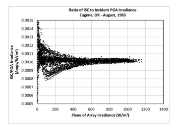
Fig. 5: Plot of ratio of short circuit current divided by the plane of array irradiance, August, 1983. (5-minute data)
