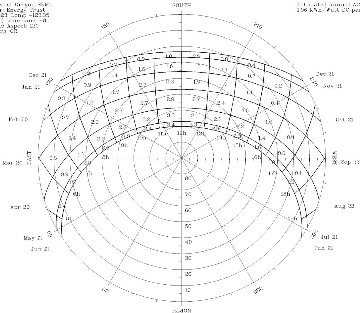
Draw the horizon on the sun path chart and shade obstructed areas. To calculate the percent reduction due to shading, enter the percentage of system power output shown on the sun path chart for areas shaded by obstructions into the table on the right.
